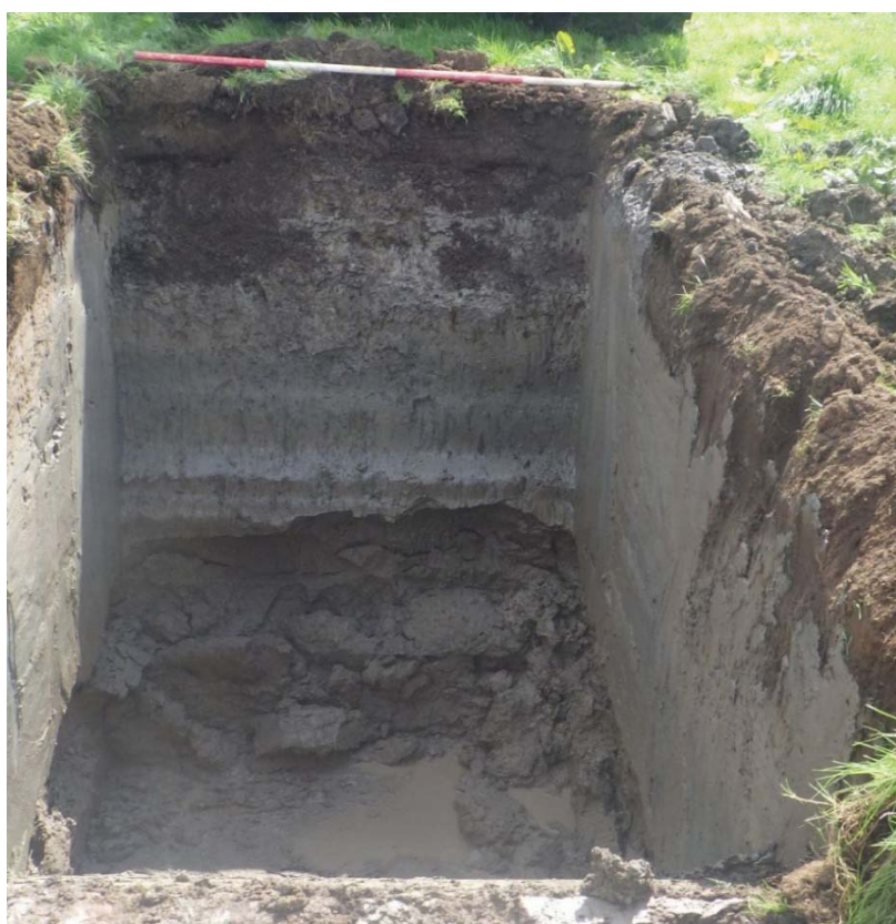
Plate 2: Topsoil over a thin layer of peat, sealing laminated alluvial and tidal-flat deposits (2m scale)
