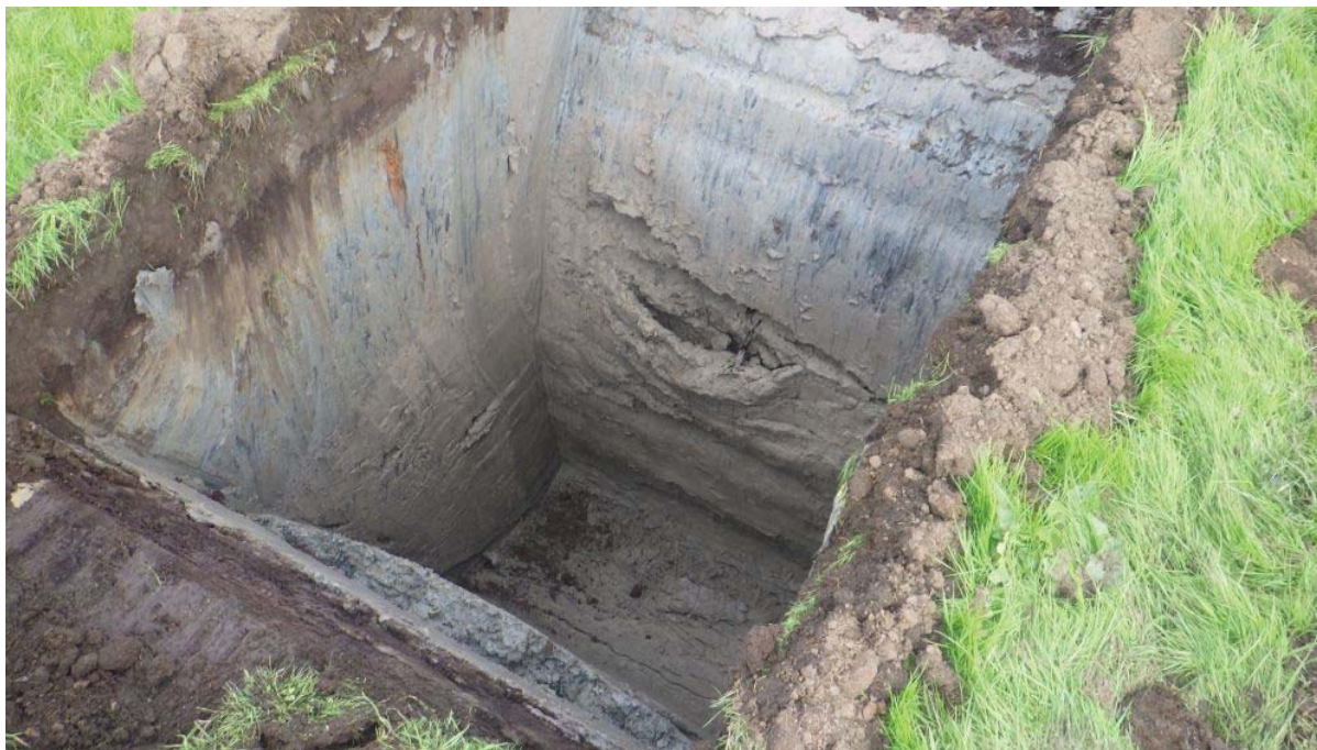
Plate 1: Topsoil over a thin layer of peat, sealing alluvium and tidal-flat deposits
