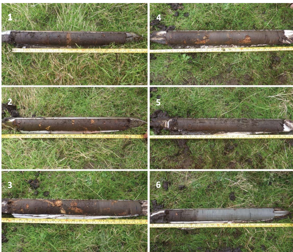
Plate 4: Trench 33: 200mm cores of peat (1-6) sealing tidal-flat deposits (6)
